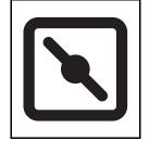
outward. Activating the choke control closes the choke plate on the carburetor and aids in starting the engine. Refer to **Starting The Engine** on page 15 of this manual for detailed starting instructions.
